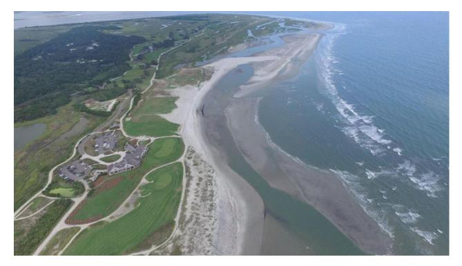
Aerial image of the completed 2015 channel relocation project in July 2015. The new inlet was opened ~3,000 ft east of the old channel.
